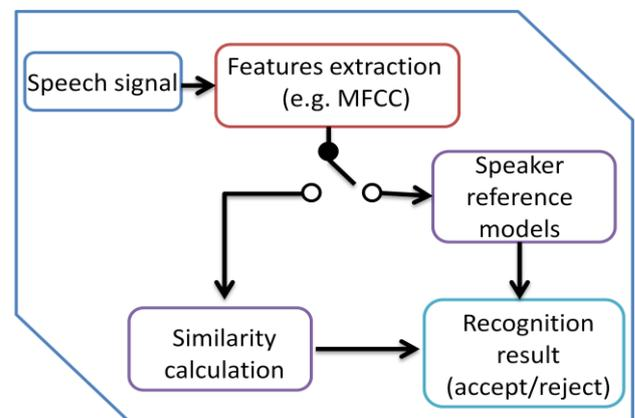
Fig. 1. Simplified block diagram for speaker recognition
