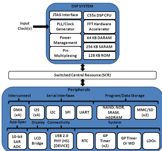
Fig. 2. Block diagram of TMS320C5515 processor (based on [9])
