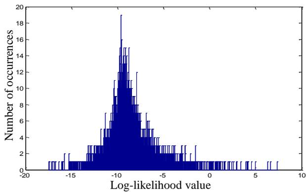
Fig. 7a. Log-likelihood distance to the correct model for 16-bit representation and GMM algorithm
