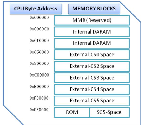
Fig. 3. Memory map of TMS320C5515 (based on [16])
