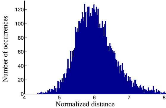
Fig. 5c. Euclidean distance to the correct model for 32-bit representation and VQ algorithm
