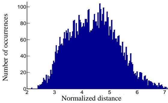
Fig. 5a. Euclidean distance to the correct model for 16-bit representation and VQ algorithm
