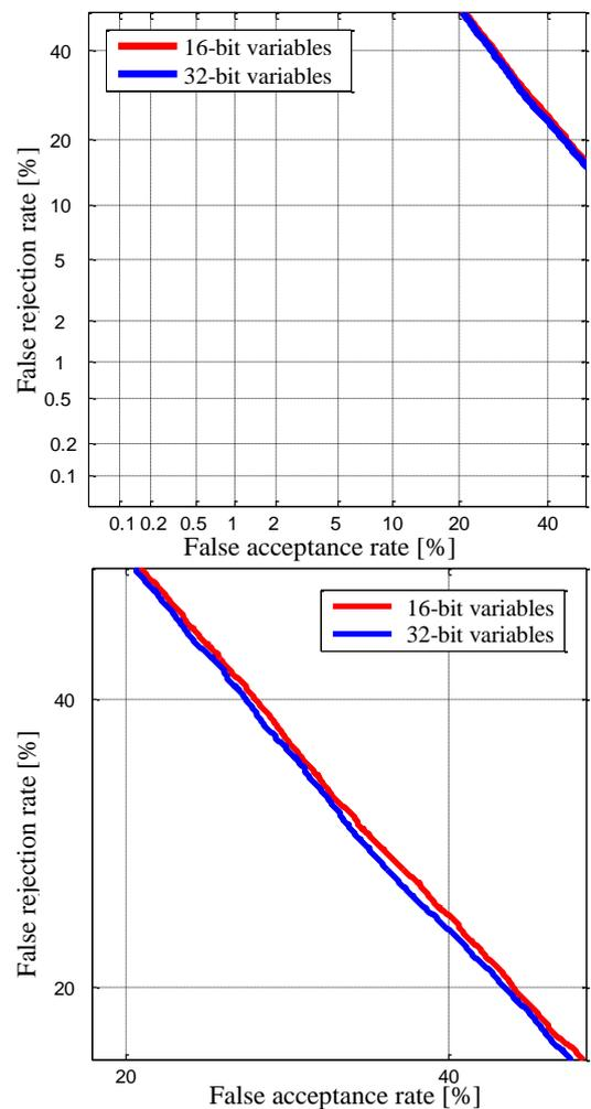
Fig. 6. FAR/FRR plots of speaker identification using Gaussian mixture models GMM (top) and its zoom (bottom)
